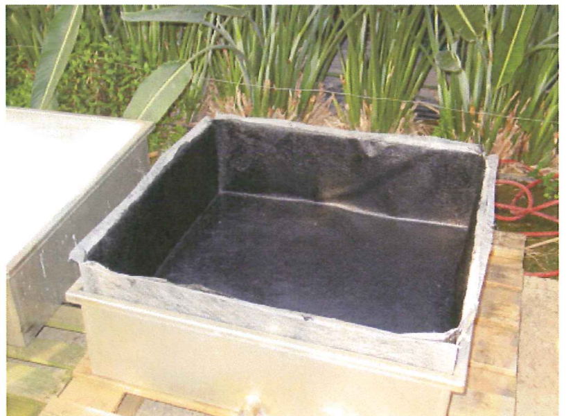
Photo 9 The test specimen has been placed on top of the protective fleece.
